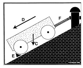
The wagon represents the femoral condyles, the inclined surface represents the tibial plateau, F =the cranial cruciate ligament, E = the medial meniscus. D = the forces of cranial tibial thrust, and C =the forces of weight.
